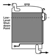
Install a 1/4 in. (6mm) diameter tube in the top fitting of the L150/EL150K1. This tube MUST EXTEND ABOVE the top tank. Form the tube into a cane so that the open end of the tube points down but still extends ABOVE the HIGHEST coolant level. The tube can be connected to the top tank if desired. Follow instructions for a PRESSURIZED SYSTEM.
